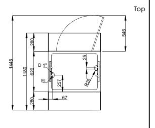
Electric Supply voltage: 220-240 V/1N ph/50/60 Hz Electrical power max: 2.32 kW Water: Drain line size: 3/4" **Key Information:** N° of doors: External dimensions, Width: 800 mm 1180 mm External dimensions, Depth: External dimensions, Height: 1304 mm Net weight: 97.5 kg Shipping height: 1334 mm Shipping width: 840 mm Shipping depth: 899 mm Shipping volume: 1.01 m<sup>3</sup>
